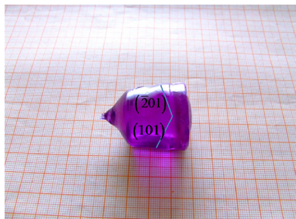
Fig. 1. NdCOB grown through the Czochralski method.
